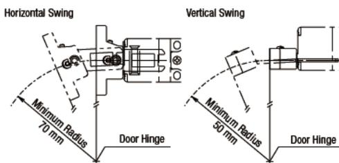
Actuator Angle Adjustment for the HS9Z-A55
