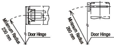
When using the HS9Z-A55 Angle Adjustable Actuator
