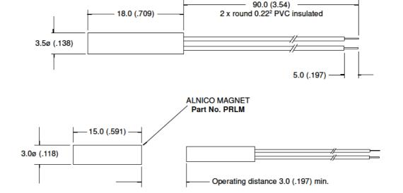
Drawings not to scale All dimensions in mm (inches) nominal Different magnets will give varying operating distances.
