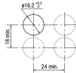
Note: Determine mounting centers to ensure easy operation.
