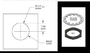
• The under panel depth for the Metal Threaded Housing configuration is 14.55 mm/(0.573 in).
