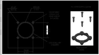
The maximum panel thickness for the Rear Mount configuration is 2.032 mm (0.08 in).
