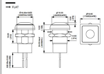
Sealed pushbutton switches ullet bushing  $\emptyset$  16 mm ullet latching
