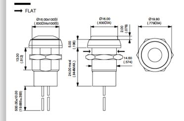
Sealed pushbutton switches • bushing Ø 16 mm • latching
